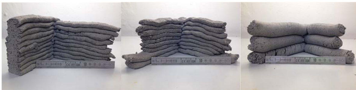
Figur 15: "hand"utskrivnen testmaterial (batteridrivnen foggistol), RISE CBI
